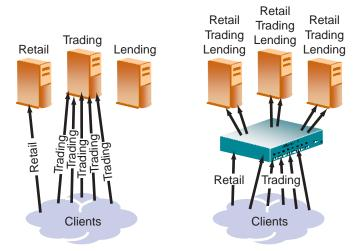
Figure 6-1 Traditional Versus SLB Network Configurations
